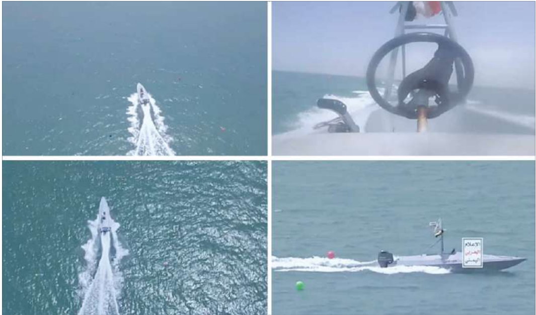
Toufan al-Mudammir with RC-controlled steering
