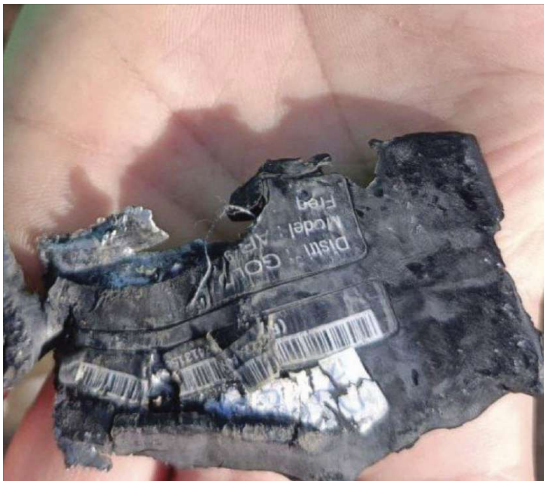
Figure 2: Pictures of the post-blast remains from pagers showing details about the company and model. (Source: X)
