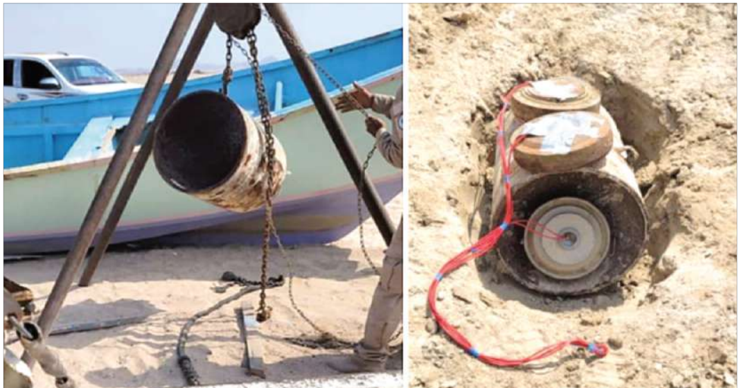
The payload (left) with an EFP warhead (right)
