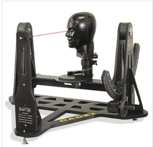
Figure 4: NIJ Static FOV apparatus – helmet fitted on a headform and tested at various angles.
