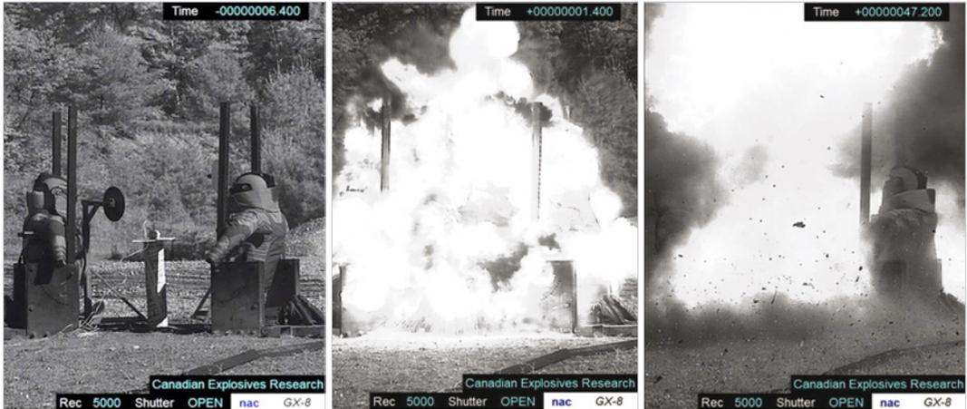
Figure 3: High speed video images of the NIJ 0117.01 blast overpressure test (0.567 kg C4 explosive, standoff 0.6 m – kneeling position). Two mannequins used for more data. Tests were conducted at the Canadian Forces Base Petawawa, under the leadership of the Canadian Explosives Research Laboratory and the supervision of Intertek auditors.
