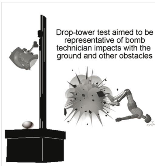
Figure 2: Helmet drop tower testing relevant to traumatic brain injury. 72 drops conducted at 3 temperatures.
