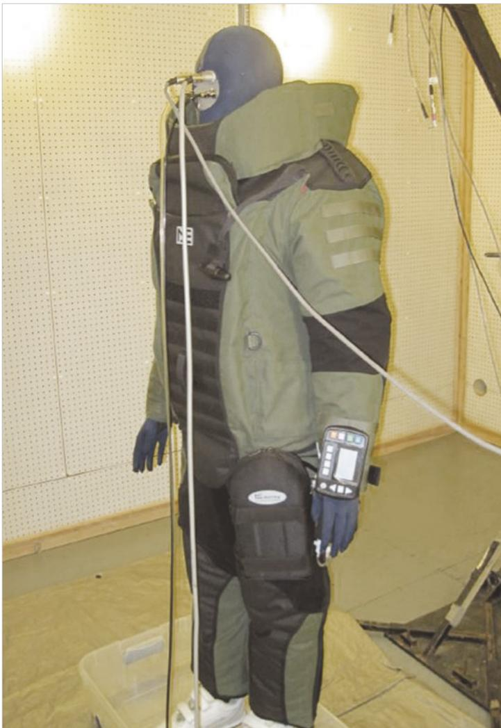
Figure 6: Personal cooling system tested in conjunction with a bomb suit against the requirements of the ASTM F2371 test methodology. Tests were conducted at the Institute for Environmental Research from Kansas State University.
