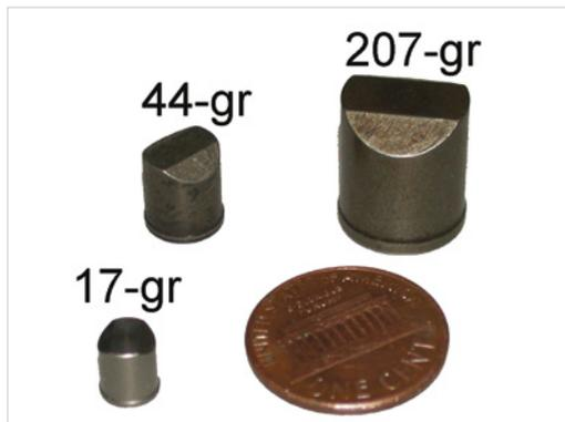
Figure 1: NIJ 0117.01 Fragment Simulating Projectiles (17, 44 and 207-grain). The large 207-grain one eliminates the need for V0 tests.
